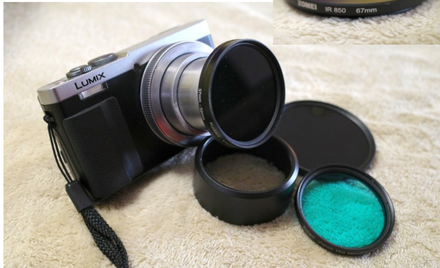
Below: Technical setup for the research on the Tilma in 2019: Full-spectrum converted Panasonic Lumix camera with strong zoom and stabilization capabilities, several filters including 720nm and 850nm infrared filters which are mounted in front of the lens via adapters. Since the environment in which the Tilma is being displayed doesn't allow the use of tripods and the 850nm infrared filter is very dark, photographing the Tilma poses an extreme challenge.
